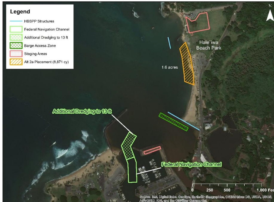
Figure A26. Alternative 2a: beneficial use of dredged material beach restoration area
